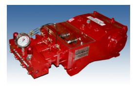
**T-300M for 15,000 PSI** - The T-300M features the "L" fluid end design, which performs at pressures from 8,000 to 15,000 PSI, and flows from 10.3 to 18.4 GPM. Four different plunger sizes allow this pump to adapt to the specific flow and pressure requirements for each job.
